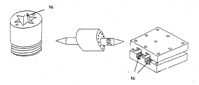
Molds for large production of pieces (when the thickness is to be reduced to allow use of less pastic material)
