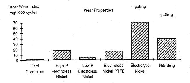
All tests were performed using a CS-10 wheel and 1000g load.
